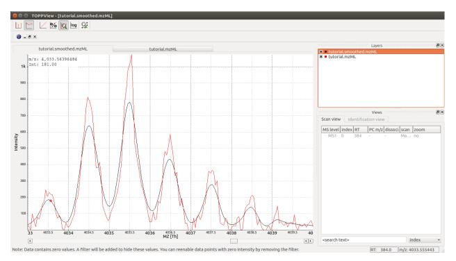
In the screenshot above we see the original data (red) and the smoothed data (black), indicating that the smoothing does clean up noise in the data significantly and will prepare the data for downstream processing, such as peak-picking.
