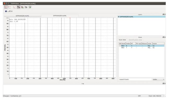
We can see all eight y ion peaks that are produced in the TheoreticalSpectrumGenerator and when we hover over one of the peaks (546 mz in this example) there is an annotation in the bottom left corner that indicates charge state and ion name ( $y_5$ + for every peak). The larger spectrum with 146 peaks can also be interactively investigated with TOPPView (the second spectrum in the file):
