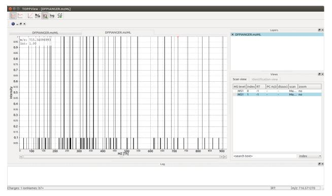
There are substantially more peaks here and the spectrum is much busier, with singly and double charged peaks of the b, y and a series creating 44 different individual fragment ion peaks as well as neutral losses adding an additional 102 peaks (neutral losses easily recognizable by their 10-fold lower intensity in the simulated spectrum).
