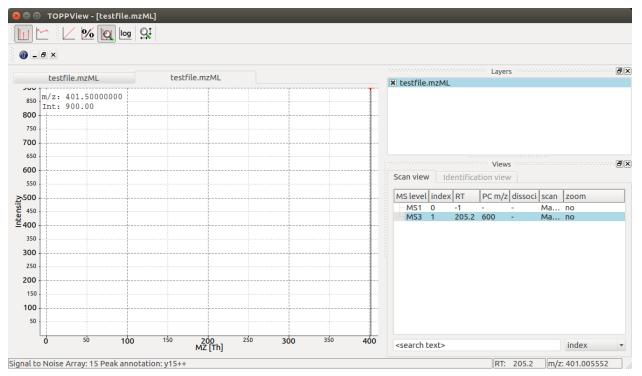
TOPPView displays our MS3 spectrum with its single peak at 401.5 m/z and it also correctly displays its retention time at 205.2 seconds and precursor isolation target of 600.0 m/z. Notice how TOPPView displays the information about the S/N for the peak (S/N = 15) and its annotation as  $y_{15++}$  in the status bar below when the user clicks on the peak at 401.5 m/z as shown in the screenshot.
